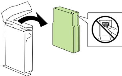
**Caution:** Do not remove any seals, or ink will leak. Do not touch the green chip on the cartridge.
